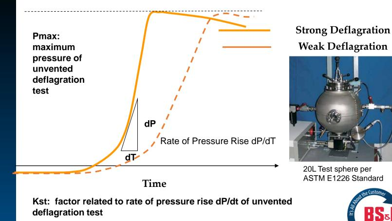
20L Test sphere per ASTM E1226 Standard
