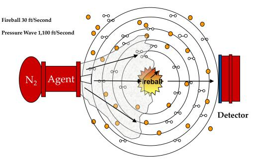
This is done using a highly sensitive & accurate pressure sensors that detects the pressure waves (1100 ft/sec) way ahead of the developing fireball (30 ft/sec) within the process and activating the Suppressing Cannons which eject the extinguishing agent, sodium bicarbonate into the process equipment to be protected and suppress the explosion by removing the heat source chemically!
